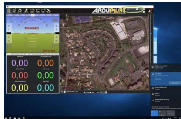
Connect Computer to hotspot, video stream will be available at rtsp://192.168.43.1:8554/fpv_stream . Open Mission planner, Set Port to "UDP", Click Connect.
