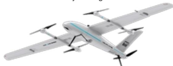
Thanks to its modular design, this VTOL can be assembled in less than a minute, without tools.
